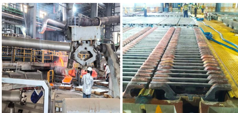
Figure 17: Anode Plate Casting and Electrolysis Circuit
